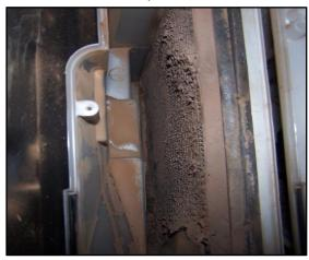
As you can see in the picture above, Dust and dirt trapped in the evaporator core is quickly turned to mud when combined with the condensation from the evaporator core. For the cost of around \$25 the cabin filter can be replaced and save you the trouble of a costly comeback!
