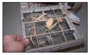
The mesh will stop leaves and large objects but will not prevent dust, dirt and grime making its way through the ducts and down to the evaporator.
