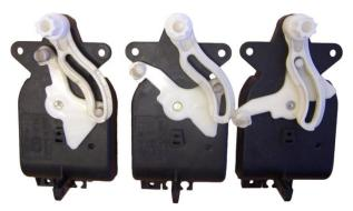
The Audi uses a stepper motor as pictured above. The error that occurs is internal to the stepper motor where by the main drive cog splits around the thin connection point at the shaft as you can see in the picture below.
